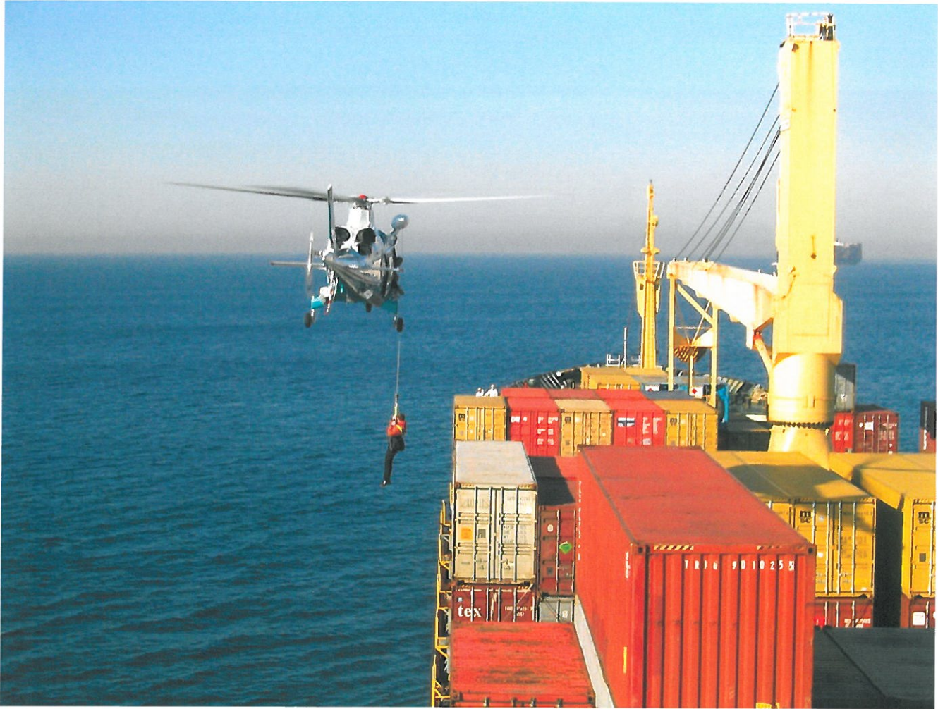
BC Coast pilots have let go of tradition and adopted helicopters for what has proven to be a safer, more cost-effective pilot transfer. Photo courtesy of the BC Coast Pilots.
